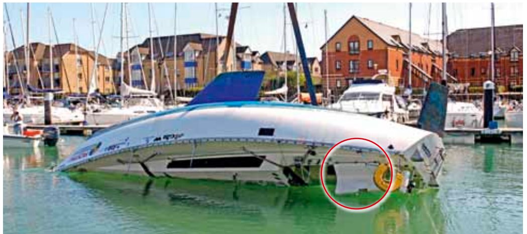
ABOVE: With no lock, the starboard cockpit locker falls open and scoops a tonne of water
