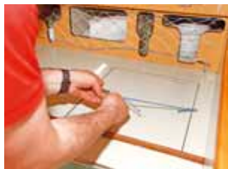
String, net and a bolt keep plates, fridge contents and stove in place
