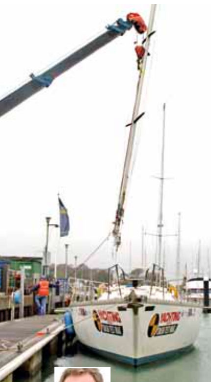
Hamble rigger Alan Moore unstepped the Crash Boat's masts at Hamble Point
