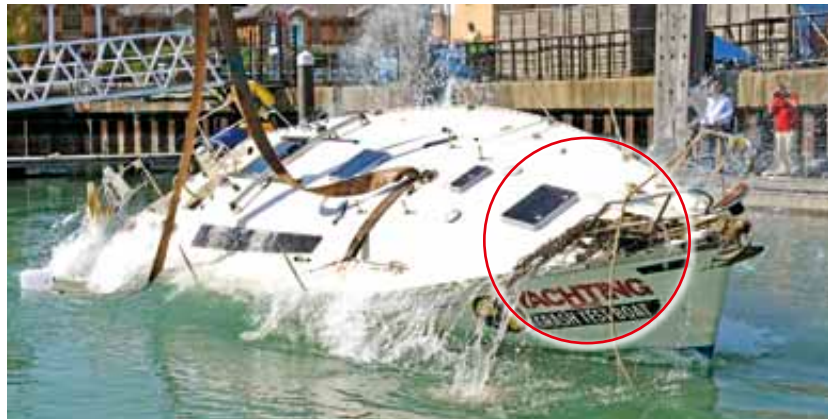
ABOVE: With no lock, the starboard cockpit locker falls open and scoops a tonne of water
