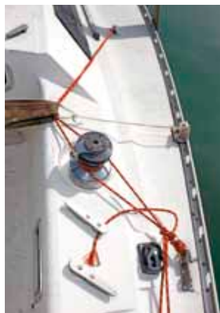
Flimsy-looking strop attachments were lashed between chainplates
