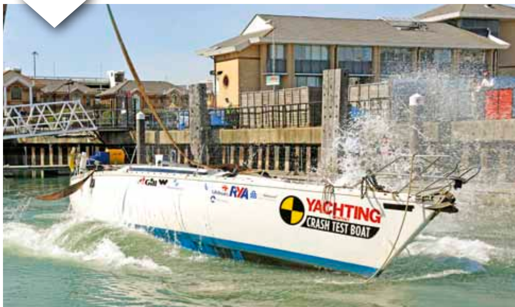
Once the keel reached around 40° from vertical, gravity took over and she slammed down dramatically
