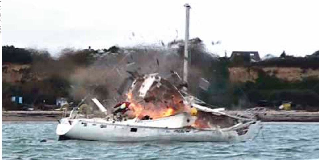
The pressure wave from the blast distorts the GRP hull of the Crash Test Boat as if it was made of rubber
