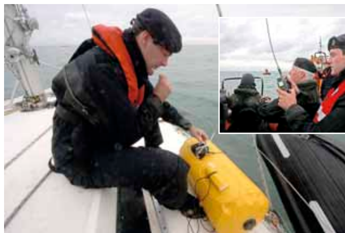
The Royal Navy’s radio-controlled detonation signal was sent by wireless remote (inset above) to a control box on a float on the yacht’s deck
