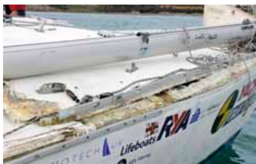
The toerail and sidedeck were ripped from the hull. The pressure wave of the blast lifted the foredeck
