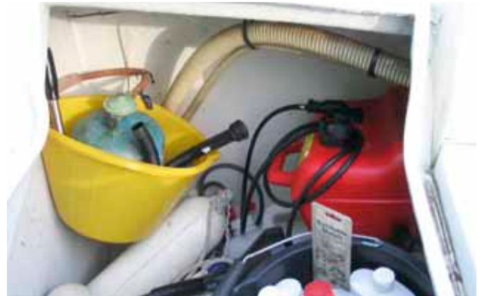
This is a dangerous installation, with the gas bottle in a bucket
