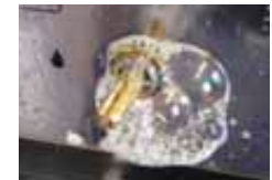
ABOVE: Soapy water will reveal leaks around the gas tap
