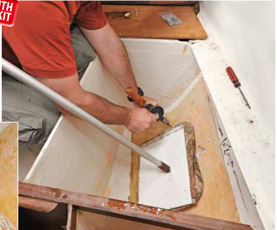
ABOVE: Drilling holes in the hull wasn't easy with a hand drill but we eventually managed it. LEFT: Self-tappers held the board well but water was beginning to 'sweat' through it
