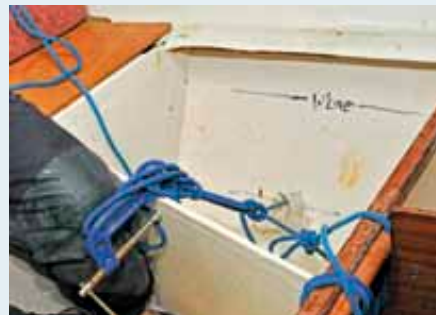
ABOVE: Kieran snagged the hauling line with a boathook and tied on the board. LEFT: Even hauled in tight, this repair leaked quite badly
