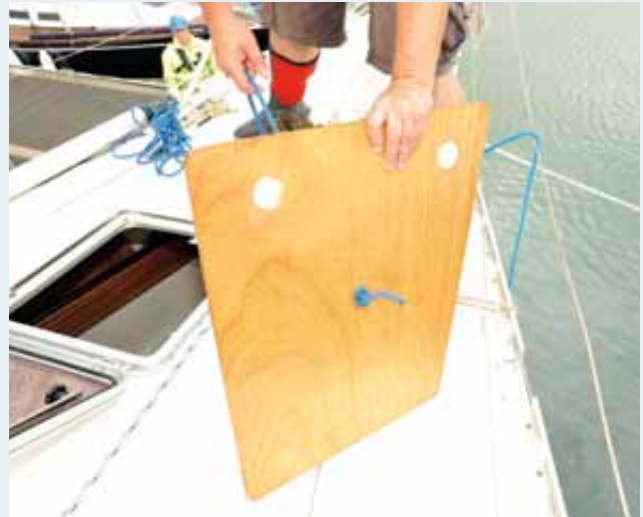
ABOVE: Kieran snagged the hauling line with a boathook and tied on the board. LEFT: Even hauled in tight, this repair leaked quite badly
