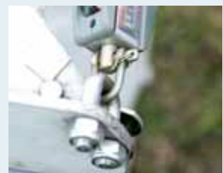
INSETS ABOVE: Vibration can cause shackles to come undone over time. Seizing them with wire or cable ties prevents it
