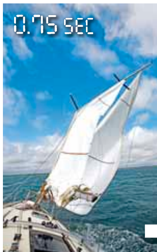
Stayed by lowers, the mast snaps...
