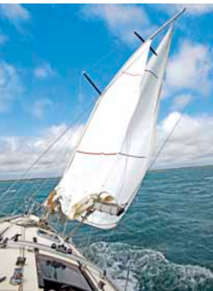
With the cap shroud and D2 free, the topmast fell away. Still stayed at the lowers, it had to break
